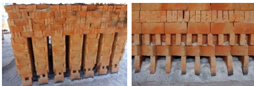
Figure 4. End-phase of the burning process with rice husk in a workshop.
