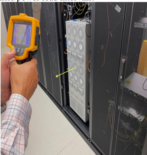
Figure 3. Using the Thermal Imaging Camera to Measure the Temperature of the Rear of the Internet Hub. The Yellow Arrow Shows the Direction of the Air Flow
