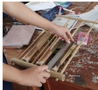
**Figure 8.** The Length Measurement of the Sound Tube
