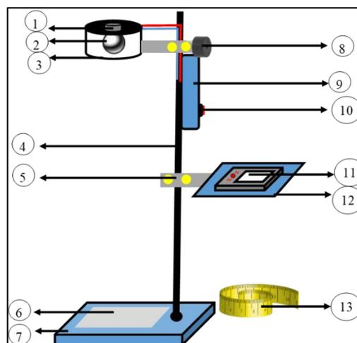
Figure 2. Design of Earth's Gravity Acceleration Detection System
