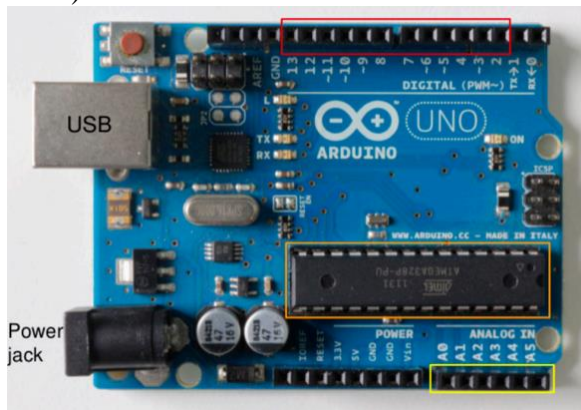
Figure 2. The Atmega328P microcontroller drives the Arduino UNO R3 hardware platform.
