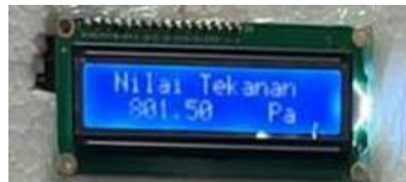
Figure 5. Hydrostatic Pressure Measurement with \Delta h of Water 8.4 cm
