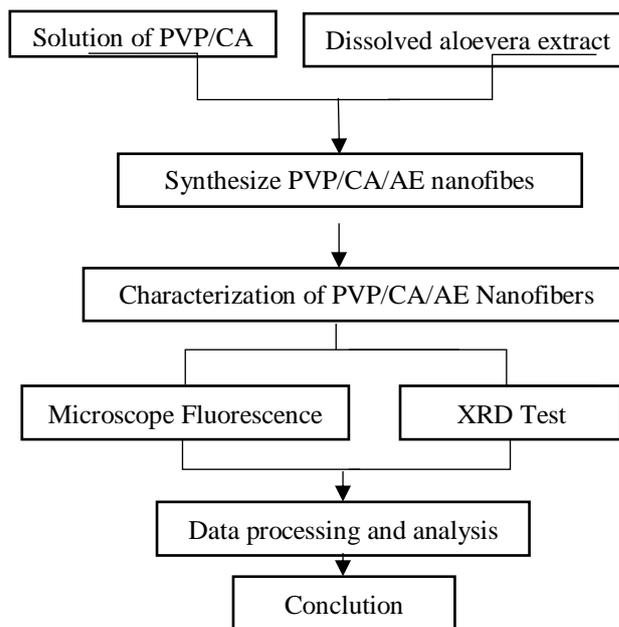
Figure 1. Experiment flowchart
