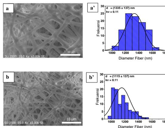
Figure 2. SEM of (a) PVP/CA and (b) PVP/CA/AE; Diameter Distribution of (a') PVP/CA and (b') PVP/CA/AE
