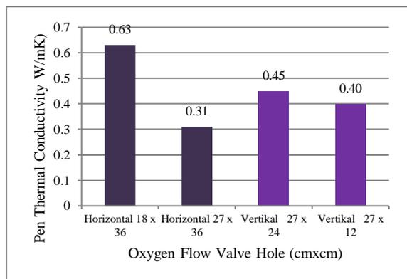
**Figure 9.** The comparison of pen thermal conductivity according to the different variations of oxygen flow valve hole
