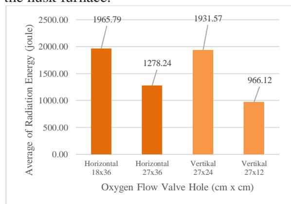
**Figure 8.** The comparison of radiation energy according to the different variations of oxygen flow valve hole
