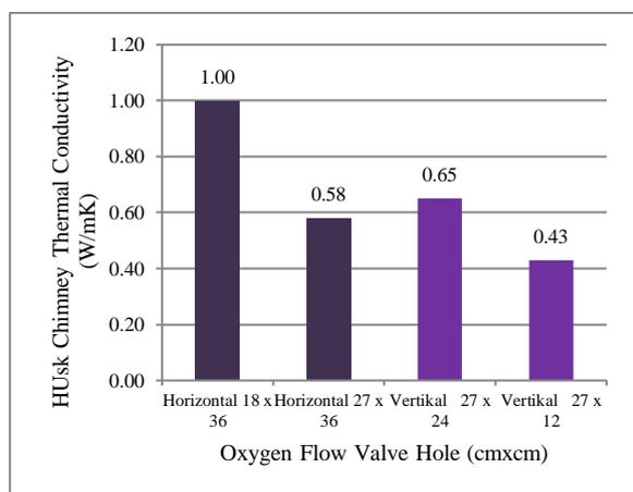
**Figure 10.** The comparison of husk chimney thermal conductivity according to the different variations of oxygen flow valve hole
