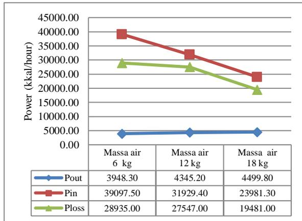
**Figure 6.** The comparison of the power input ( $p_{in}$ ), power output ( $p_{out}$ ), and power loss ( $p_{loss}$ ) according to the difference in mass variation of heated water
