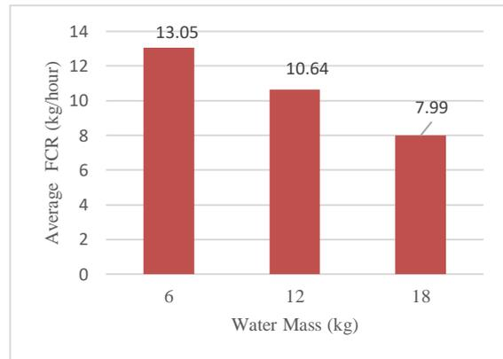
Figure 2. The comparison of average FCR according to the difference in mass variation of heated water
