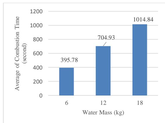
Figure 3. The comparison of average boiling time according to the difference in mass variation of heated water
