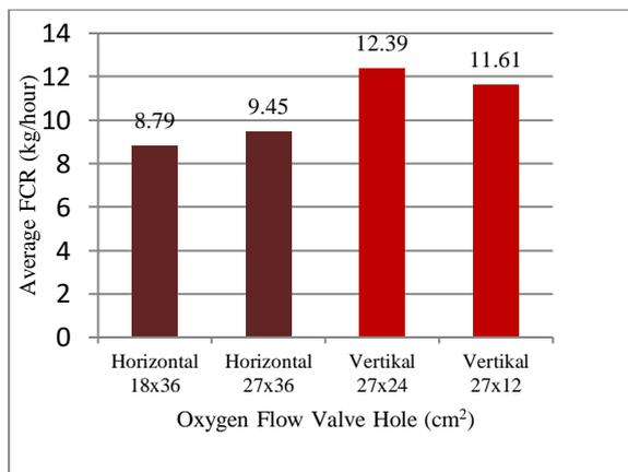
Figure 4. The comparison of average FCR based on the different variations of oxygen flow valve hole
