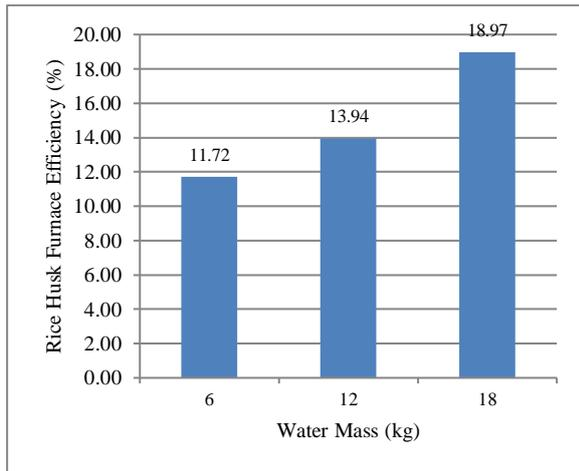
**Figure 11.** The comparison of husk furnace efficiency according to the difference in mass variation of heated water
