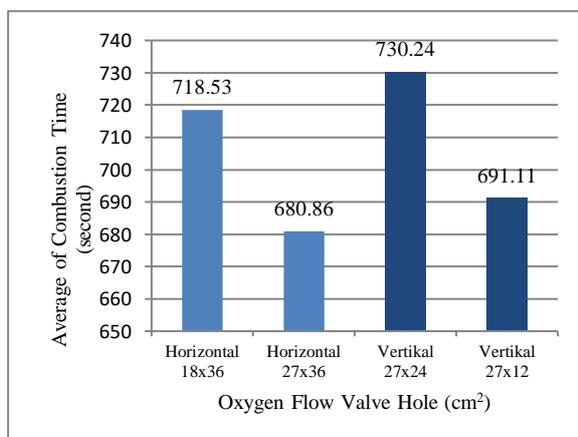
Figure 5. The comparison of the average of the boiling time based on the different variations of oxygen flow valve hole
