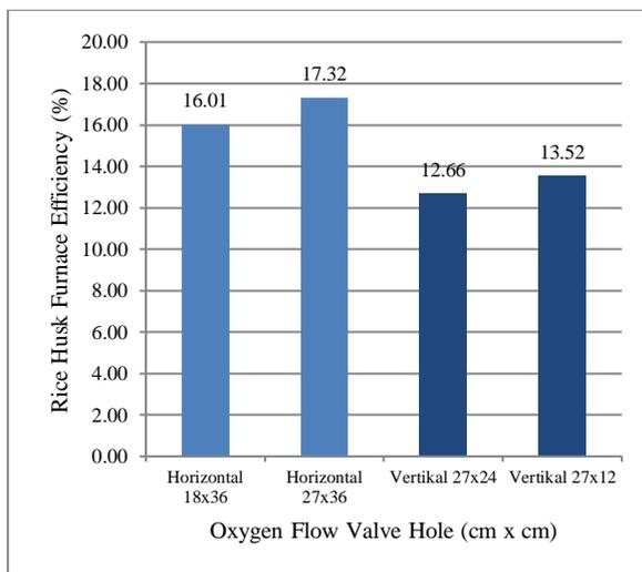
**Figure 12.** The comparison of husk furnace efficiency according to the different variations of oxygen flow valve hole
