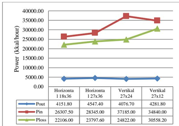
**Figure 7.** The comparison of the power input ( $p_{in}$ ), power output ( $p_{out}$ ), and power loss ( $p_{loss}$ ) according to the different variations of oxygen flow valve hole
