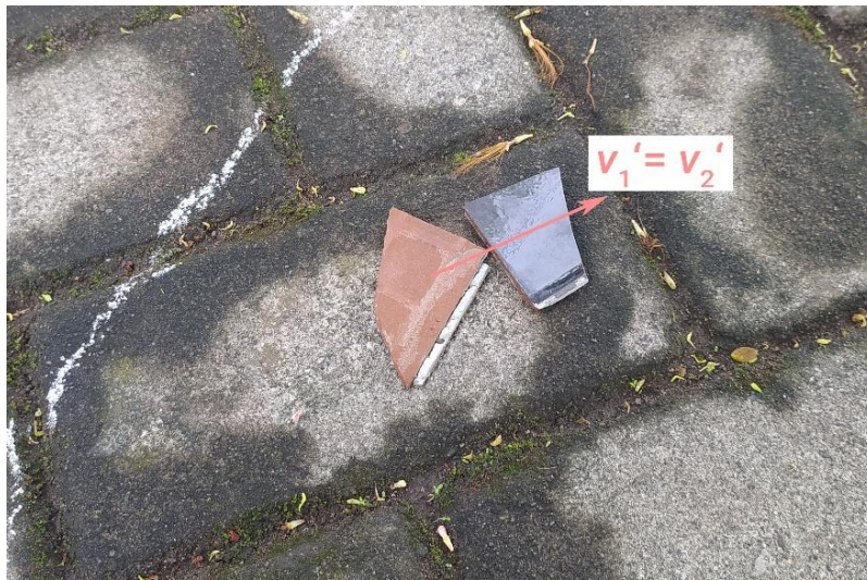
Figure 8. The condition of two gacos after the collision has the same final velocity because the type of collision is not elastic at all.
